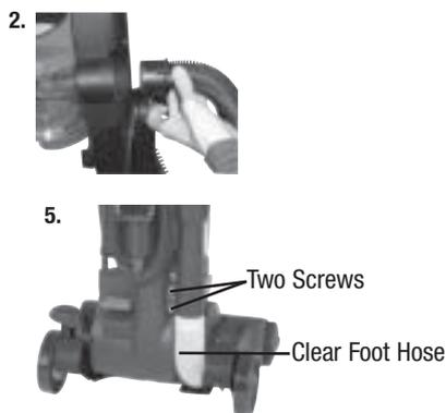
**\*Note: If the debris cannot be reached through the hose, then follow the instructions for cleaning the air passageway in the "Clean and replace rotating floor brush" section.**
